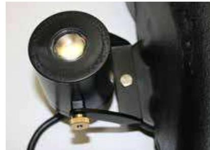
5. Install the 1/4" Flat Washer, 1/4" Lock Washer and 1/4" Nut against the underside of the float tab as shown in Figure 5. Tighten the nut until snug using the 7/16" Wrench.
