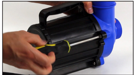
Step 12: Re-fit all four screws around the impeller housing and tighten up.
